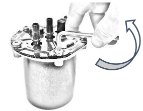
3. Unscrew and dispose the old screws.
