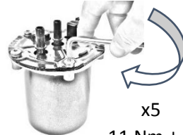
12. Tighten the new screws supplied with the new element. x5 11 Nm ± 1
