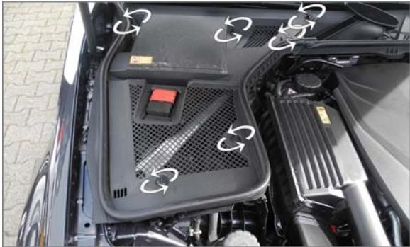
**EN** Open the front bonnet. Turn the filter frame holders 45 degrees to the left
