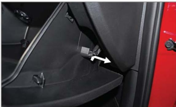
(EN) Remove the protecting device.
