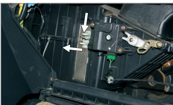
**EN** Carefully remove the first filter, the second one will slide downwards
