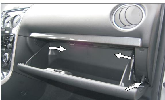
**EN** Remove the glove compartment
