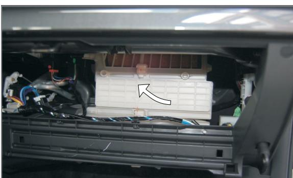
**EN** Remove the filter housing
