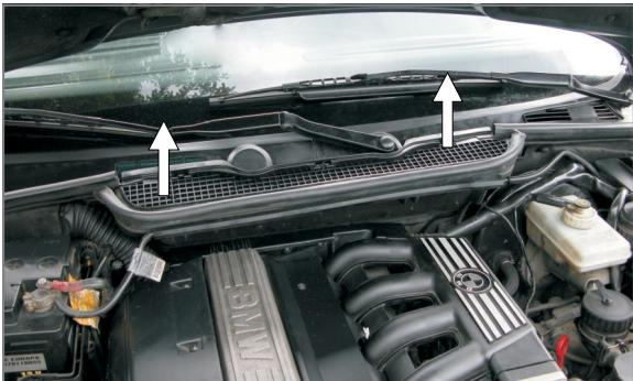
(EN) Remove the rubber seal. Remove the screen segment
