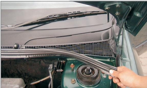
**EN** Remove the rubber seal
