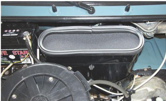
(EN) Remove the rubber seal
