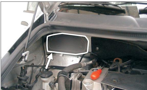
**EN** Remove the protecting device
