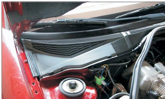
**EN** Remove the rubber gasket and open the cover of the filter chamber
