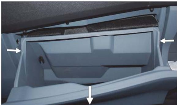
**EN** Open the glove locker, remove the glove compartment
