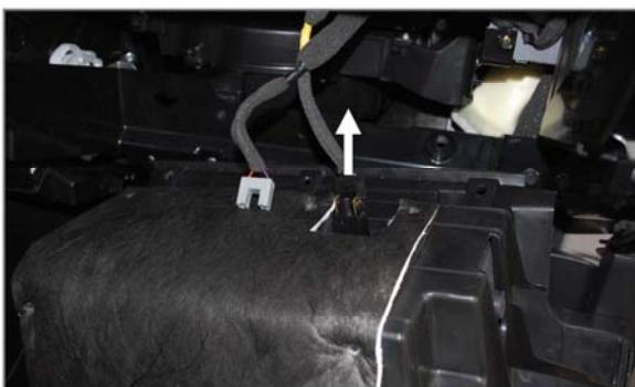
(EN) Disconnect the electric circuit
