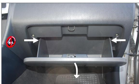
(EN) Remove the glove compartment
