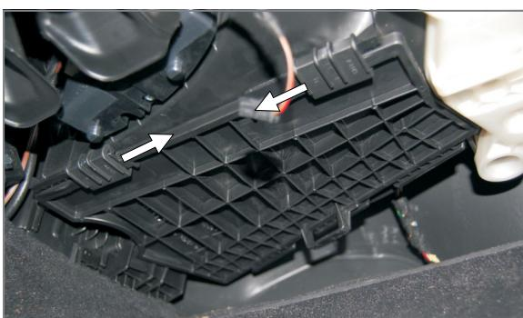
(EN) Move sideways the locks, which hold the cover of the filter chamber, remove the cover of the filter chamber
