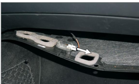
(EN) Disconnect the electric circuit, remove the upholstery panel
