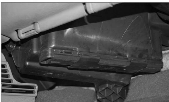
(EN) Remove the filter fastener, remove the old filter, insert the new one and carry out the opposite to all the previous operation at the reversed order
