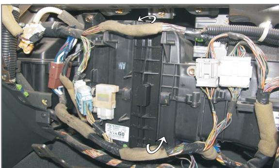
**EN** Remove the filter housing
