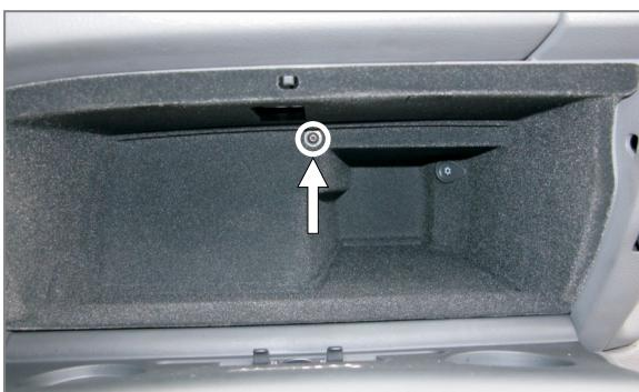
**EN** Loosen the screw and remove housing
