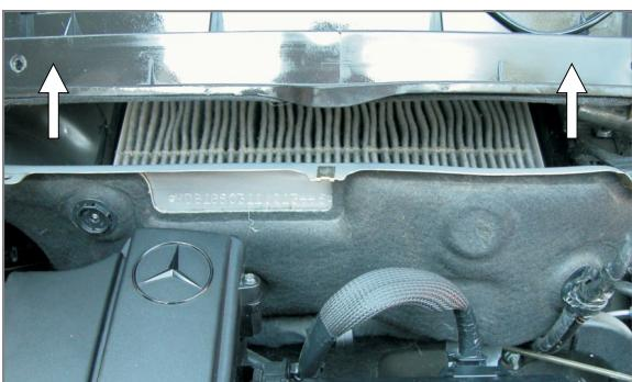
EN Carefully lift and remove the cover
