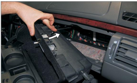
**EN** Disconnect the electric circuit
