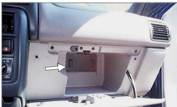
**EN** Open the glove compartment, the filters are located behind the rear wall of the compartment
