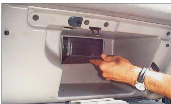
**EN** Remove the cover of the filters chamber
