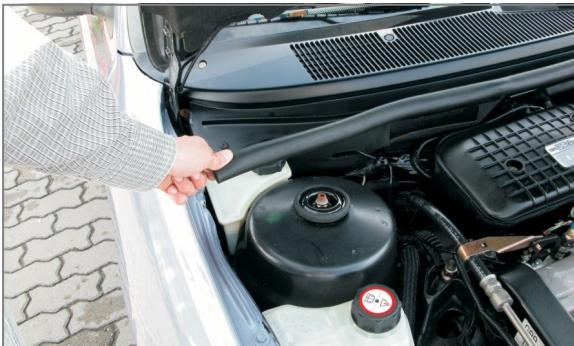
**EN** Remove the rubber seal
